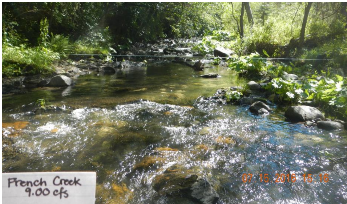
Photo 16. Post-lease streamflow measurement on French Creek recorded 9.00 cfs.
